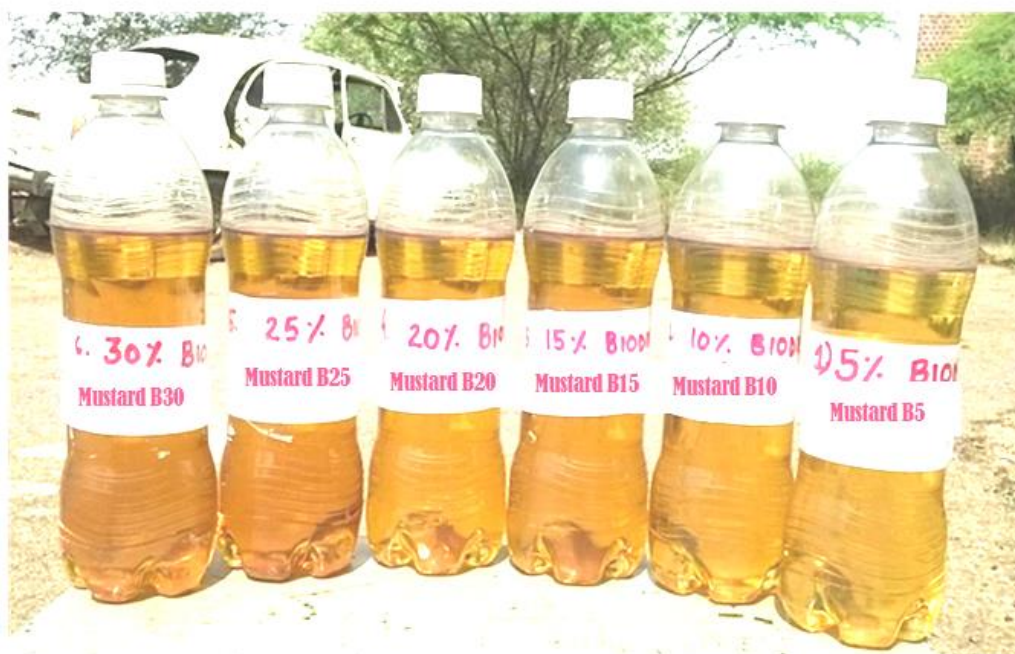
Figure 2. Sampling of Mustard Biodiesel blending with diesel
