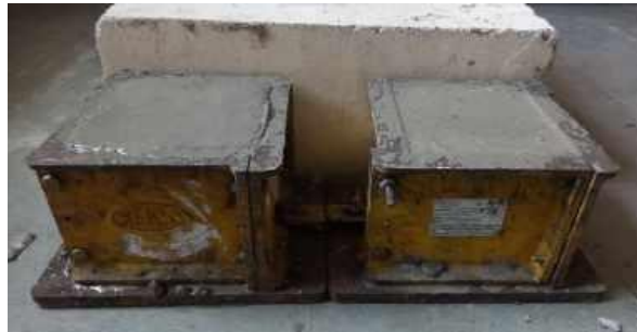
Figure.3. Concrete mix poured into molds to set
