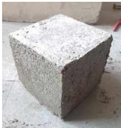
Figure5. Concrete cube placed out of water for few hours to dry before testing
