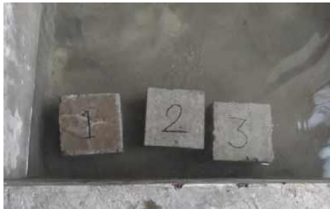
Figure4. Concrete cubes placed into water for curing
