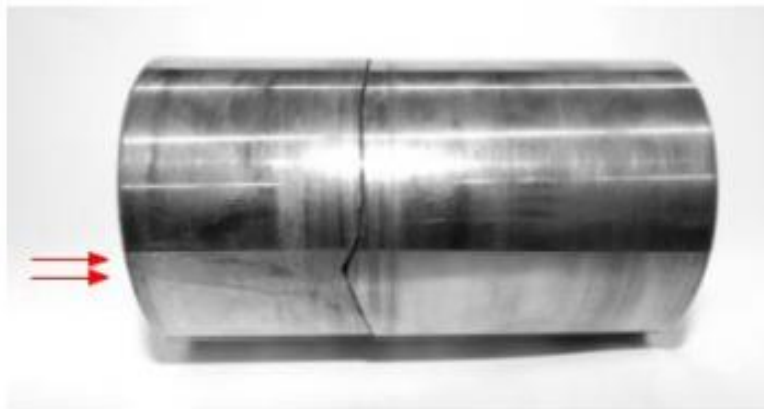
Figure 5. Circumferential crack in piston pin [1]
