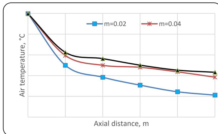
Figure 10: Effect of mass flow rate on outlet temperature of EATHE
