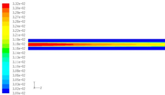
Figure 4: Temperature variation contour for Full length of buried pipe
