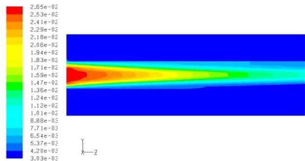
Figure 5: Temperature variation contour in buried pipe
