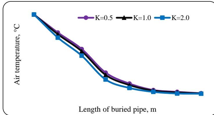
Figure 9: Effect of thermal conductivity of soil on performance of EATHE
