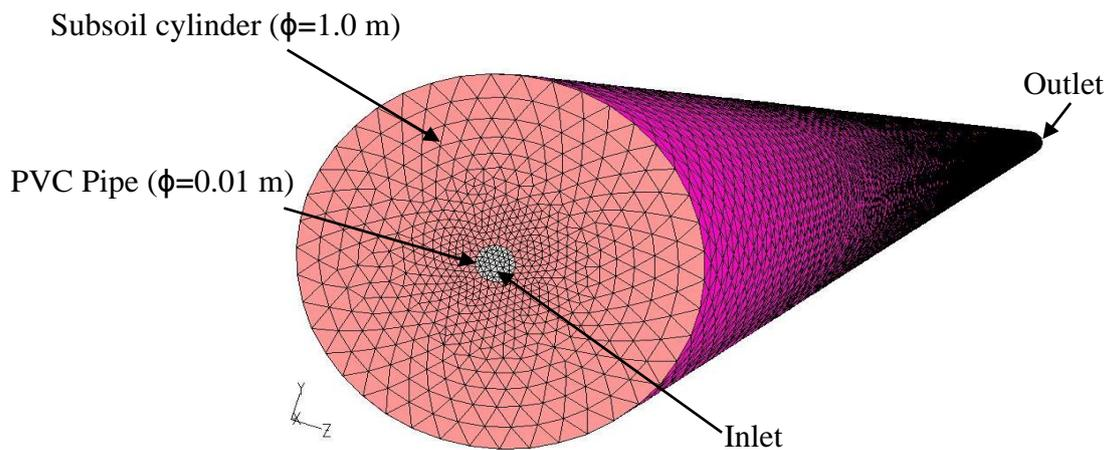
**Figure 1.** CFD geometry and Meshing of EATHE system
