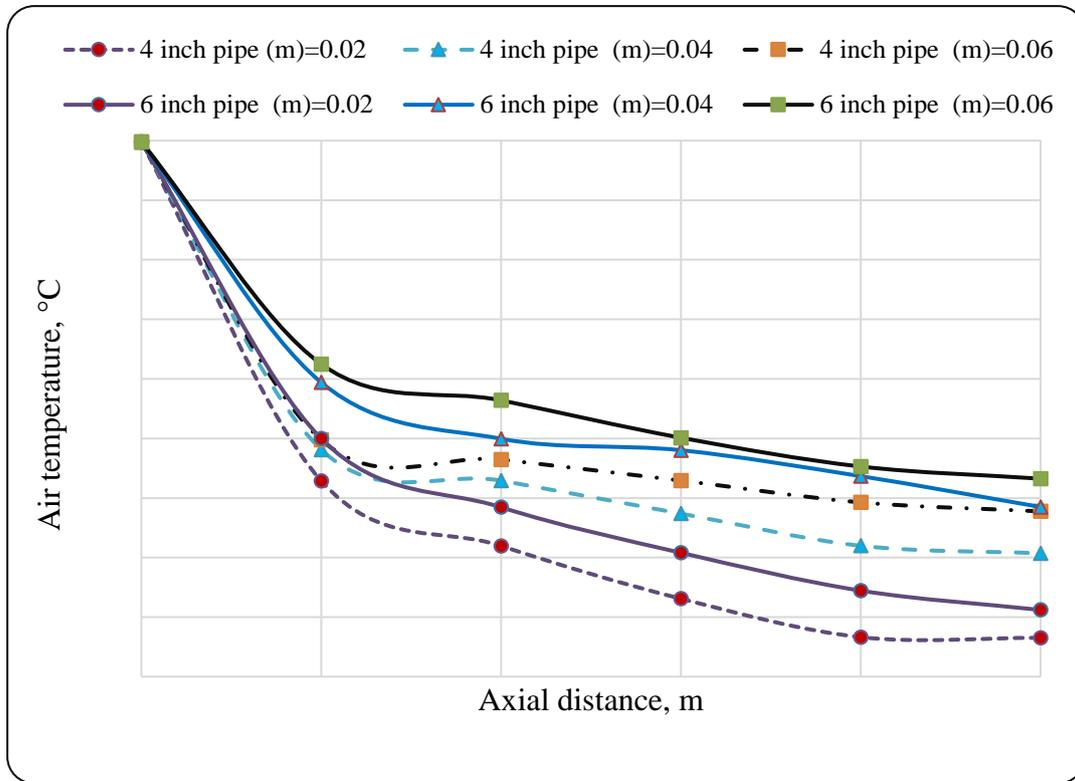
**Figure 11:** Effect of diameter at different mass flow rate on outlet temperature of EATHE
