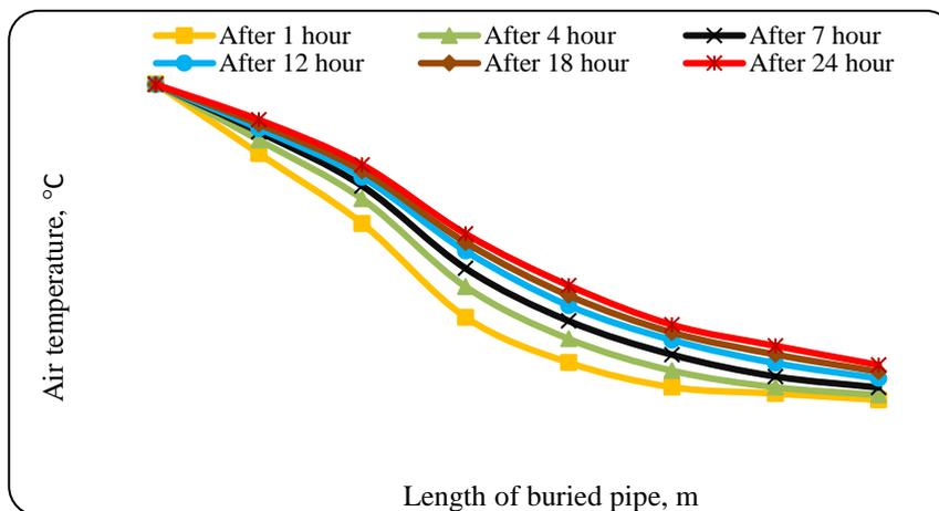
Figure 8: Effect of running time on EATHE performance
