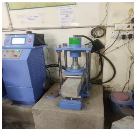
Figure 8. Flexural Test being conducted
