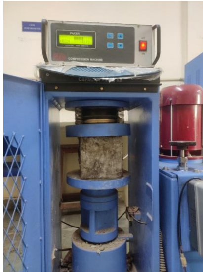
Figure 6. Compressive Test being conducted
