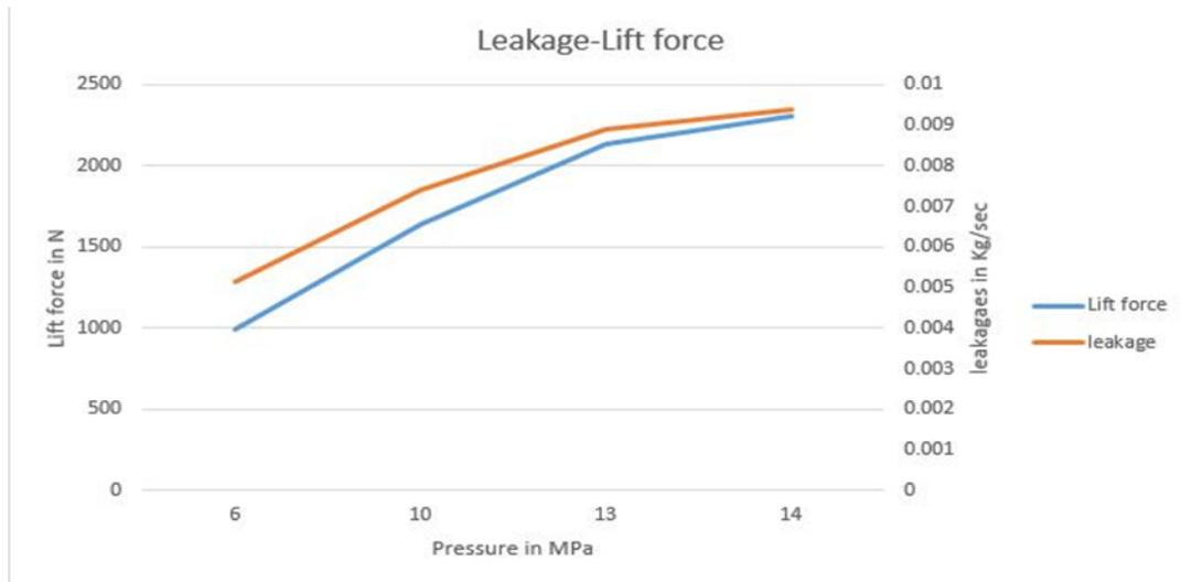
**Figure 13:** Effect of pressure variation on Lift and leakage
