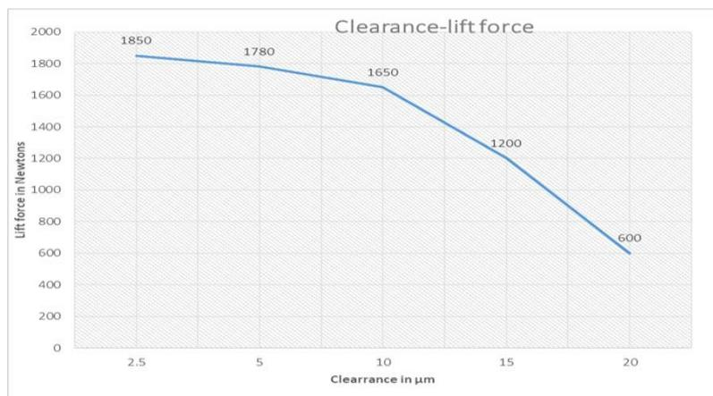
Figure 19. Variation of lift force with clearance.
